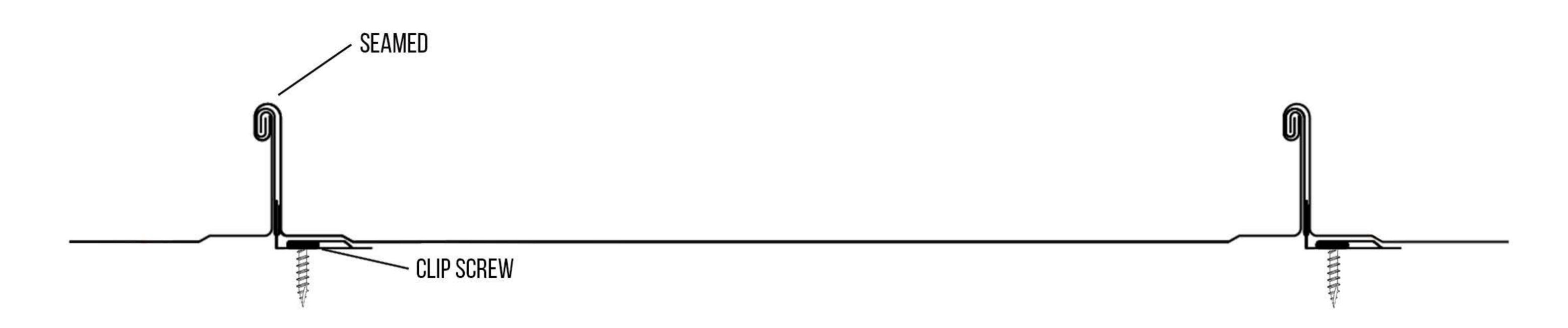
ONCE PANEL IS PLACED, SPACE CLIPS 24" O.C. AND FASTEN USING 1" CLIP SCREW OR DESRED SCREW PER APLICATION. AFTER THE SECOND PANEL IS PLACED OVER FIRST PANEL AND CLIP, IT IS OKAY TO HAND SEAM THESE PANLS TOGETHER. ONCE THE ROOF IS HAND SEAMED AT EAVE AND RIDGE, IT WILL THEN NEED TO BE MECHANICALLY SEAMED USING PROVIDED SEAMER.
